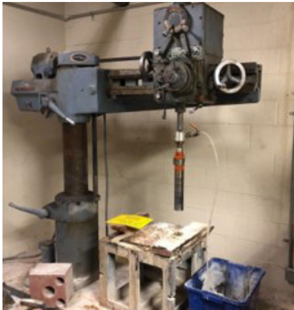
Rock Coring for Hard Rock specimen Preparation
